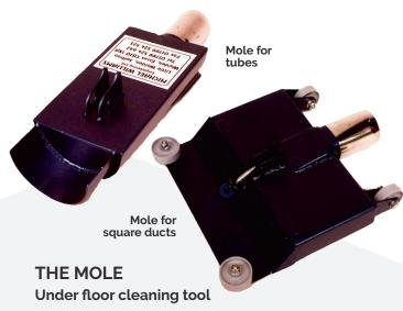
The Mole is designed to clear between the laterals of drying floors in grain stores. By connecting the Mole to the Big Brute vacuum cleaner pipe, it can be pushed through the offending under-floor corridor with the use of drain rods, clearing the way as it goes.
